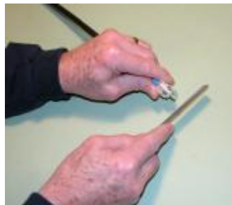
Step #12 File off the rough end of the centre conductor
