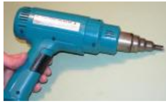
Step #11A Use a good quality heat gun to shrink the tubing. Be careful not to apply too much heat. See note below about the heat gun
