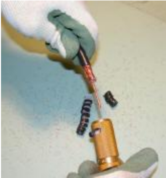
Step #5 The jacket has been fully trimmed off
