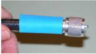
Step #11 Slip the piece of 3/4" shrink tubing into place
