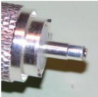
Step #12 C The finished job with a little of the centre conductor showing beyond the connector
