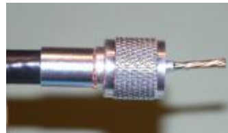
Step #9 After the solder has cooled, slip the barrel up to
