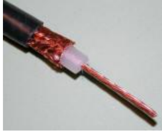
Step #6 Using very sharp nippers, carefully trim back about 1/4" of the braid
