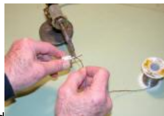
Step #8 Hold the assembly on a slight angle to solder the centre conductor. While you can crimp the centre conductor, a better mechanical connection is made if it's soldered. It helps to have a vise or support for the soldering iron.
